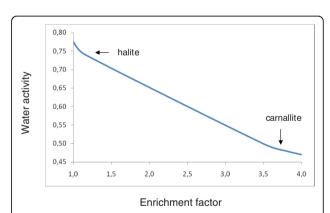
**Figure 1 Water activity changes for isothermal evaporation of Urmia Sea water at 25°C.** The initial precipitation points of halite and carnallite, computed in accordance to the Pitzer approach are indicated.
