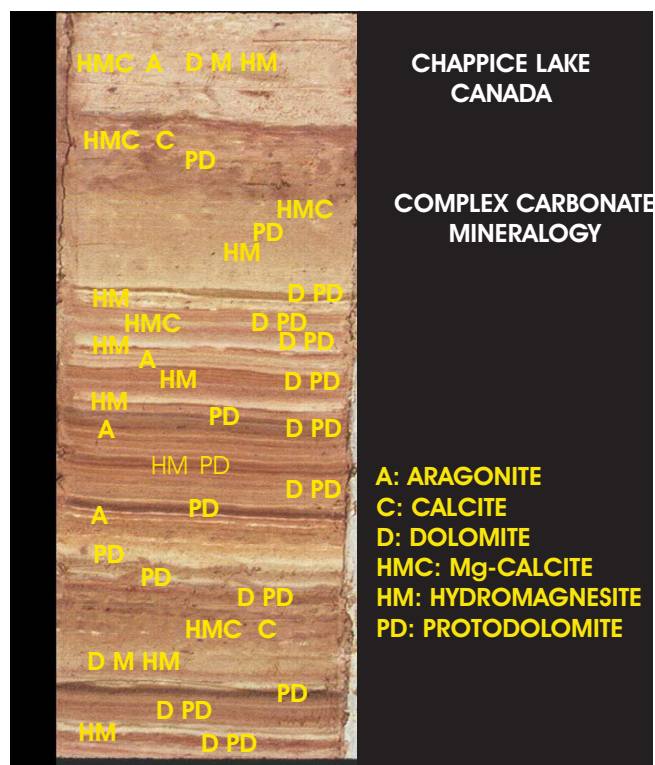
Figure 22 Chappice Lake laminated carbonates. Photograph of a section of core from Chappice Lake showing the fine lamination and the complex carbonate mineral assemblage present in this otherwise relatively simple playa basin; modified from [10, 59].
